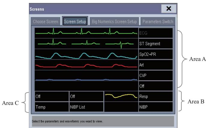
The ECG parameter and the first ECG waveform always display in the first row. The configurable areas can be classified as Area A, Area B, and Area C.
